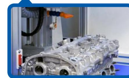
The work surface is 1100x770mm and comes in hardened anodized aluminium. The surface is perforated for ease in positioning pieces and speeding up the pre-marking process.
