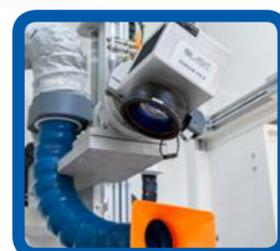
Operator use is minimized since the machine can run on automatic during 90% of the workflow. The Z axis allows marking individual pieces with a thickness ranging from 0 to 450 mm. **The work surface is 750x480 mm** and comes in hardened anodized aluminium. The surface is perforated for ease in positioning pieces and speeding up the pre-marking process.
