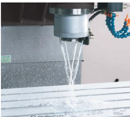
Coolants Jets Around Spindle
