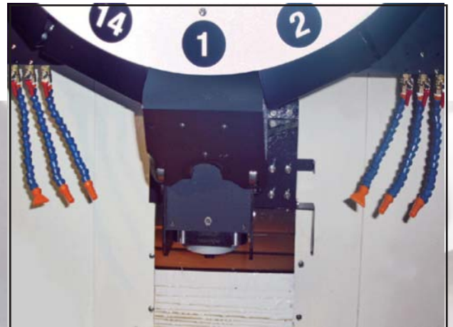
MULTIPLE COOLING DEVICES IMPROVE PROCESSING EFFICIENCY (COOLANT X 4, AIR X 2)
