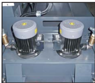
TWO COOLANT PUMPS
