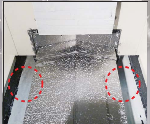
SPECIAL DESIGNED CHIP OUTLET FOR CHIP REMOVAL.
