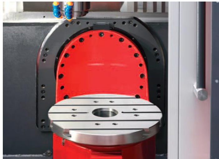
Swivel-rotary table. The swivel-rotary table has a flexible clamping surface with a diameter of 400 mm and can be loaded with 80 kg. A workpiece with a maximum edge length of 250 x 250 x 225 mm can be processed on 5 sides with optimum results.
