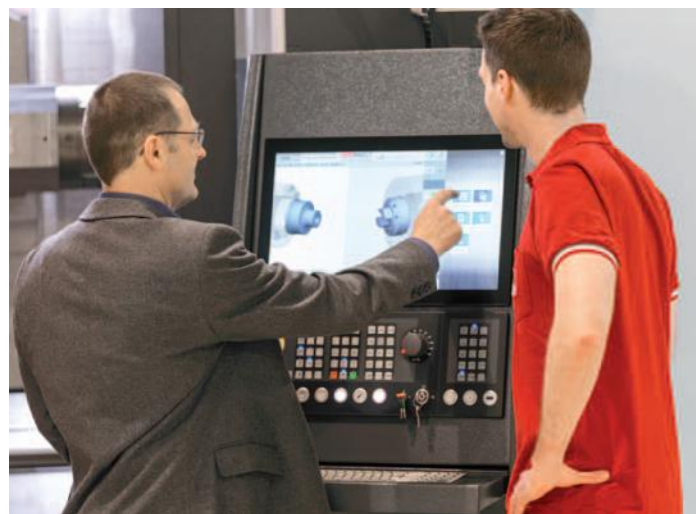
emcoNNECT's hardware basis is a 22" industrial touch control panel combined with an industrial PC (IPC).
