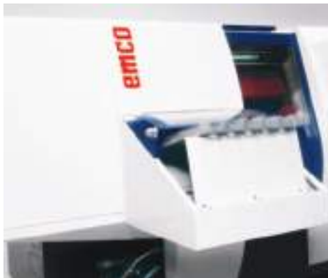
Multiple infeed chutes for loading rotationally symmetrical blanks. A sensor monitors the availability of blank parts for each infeed chute.
