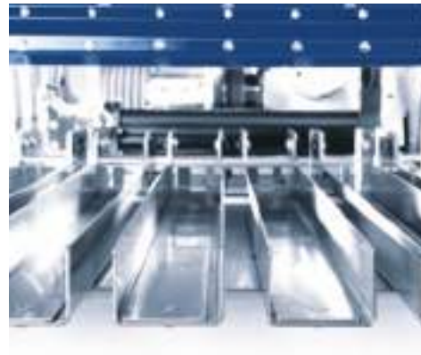
Multiple infeed chutes for loading rotationally-symmetrical blanks. The length of the blanks determines the number of infeed chutes.
